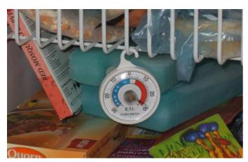
This easy to read fridge/freezer thermometer has a  $\emptyset$ 52 mm dial. The thermometer indicates temperature over the range of -30 to 30 °C in 1 °C divisions.
